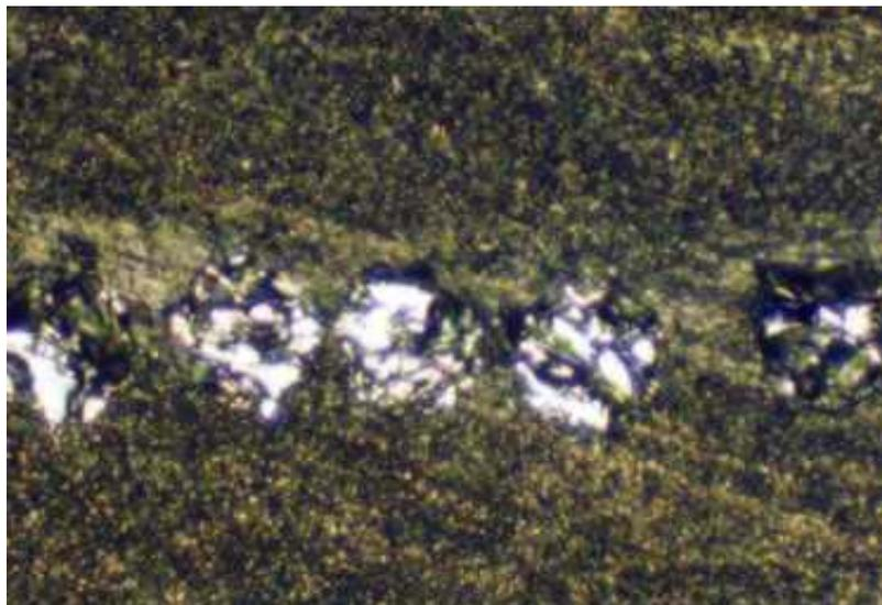
**Figure 3-4b** Medium grit diamond cut for boron graphite composite.
