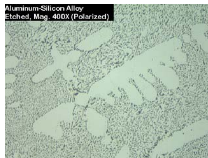
Figure 4. Aluminum-silicon alloy solidification microstructure
