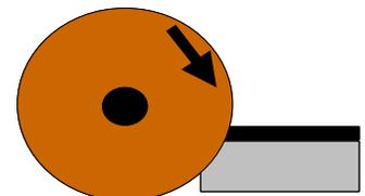
Cut through the smallest cross section and orient sample so that coatings are kept in compression during sectioning.
