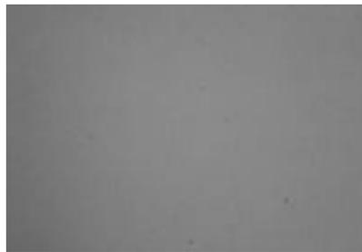
Silicon Nitride—Polished with 6, 1  $\mu\text{m}$  diamond and colloidal silica, 5 minutes each step)
