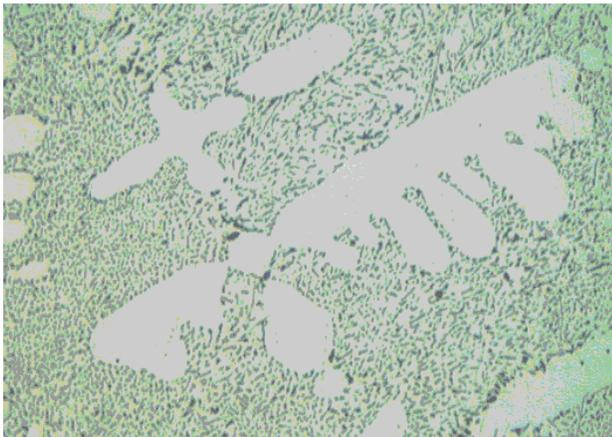
Polishing of aluminum-silicon alloy with Nanometer alumina
