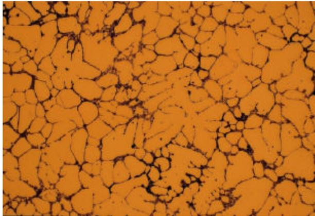
Polishing of copper alloy with Nanometer alumina
