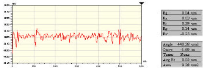
Surface roughness of a low carbon steel polished with 3 um polycrystalline diamond
